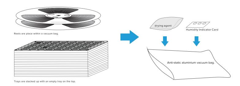
The vacuum bag is placed inside the box and a Model Name Label stuck on the front-side of each box.
